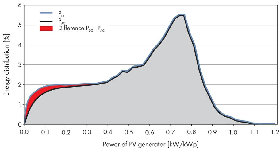
Figure 6: Efficiency, input power and output power of the inverter when the nominal power of the inverter is more than 100% of the PV array power
