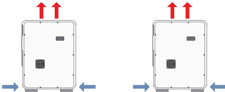
Figure 9: Arrangement of actively cooled inverters to optimize heat dissipation: Sunny Tripower CORE1 / CORE1-JP / CORE1-US
