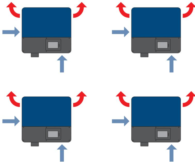
Figure 8: Arrangement of actively cooled inverters to optimize heat dissipation: STP XXXXXTL-30
