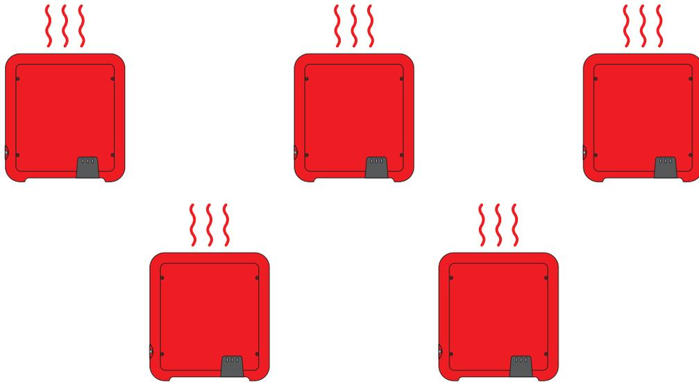
Figure 7: Arrangement of passively cooled inverters to optimize heat dissipation: SBxx-1AV-40
