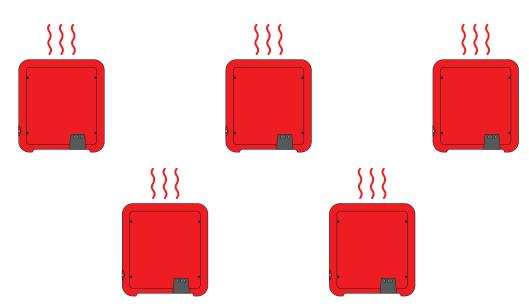
Figure 7: Arrangement of passively cooled inverters to optimize heat dissipation: SBxx-1AV-40
