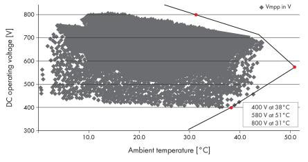
Figure 3: Operating points of a PV system and characteristic curve of the operating range within which the inverter can feed maximum power into the grid (location of the PV system: Australia, Alice Springs; 140% oversizing)
