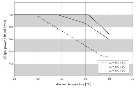
Figure 2: Example for derating behavior of an SMA inverter at various operating voltages
