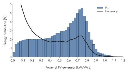
Figure 4: Energy supply relative to the power range of the PV array (example: Freiburg im Breisgau, Germany)
