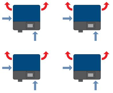
Figure 8: Arrangement of actively cooled inverters to optimize heat dissipation: STP XXXXTL-30
