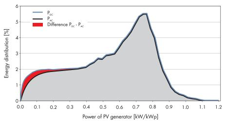
Figure 6: Efficiency, input power and output power of the inverter when the nominal power of the inverter is more than 100% of the PV array power
