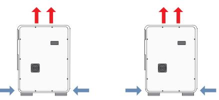
Figure 9: Arrangement of actively cooled inverters to optimize heat dissipation: Sunny Tripower CORE1 / CORE1-JP / CORE1-US
