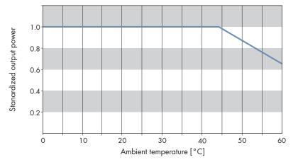
Figure 1: Example of a power curve with temperature derating
