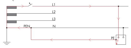
Example: Disconnection through circuit breaker in case of fault in the TN-C-S grid configuration
